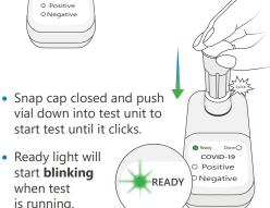
If Ready light is not blinking within 5 seconds, use palm of your hand to push down more firmly to start test.
